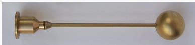
Figure 1: One of the two Langmuir probes from the Swedish institute of Space Physics in Uppsala on board ESA's space vehicle Rosetta
